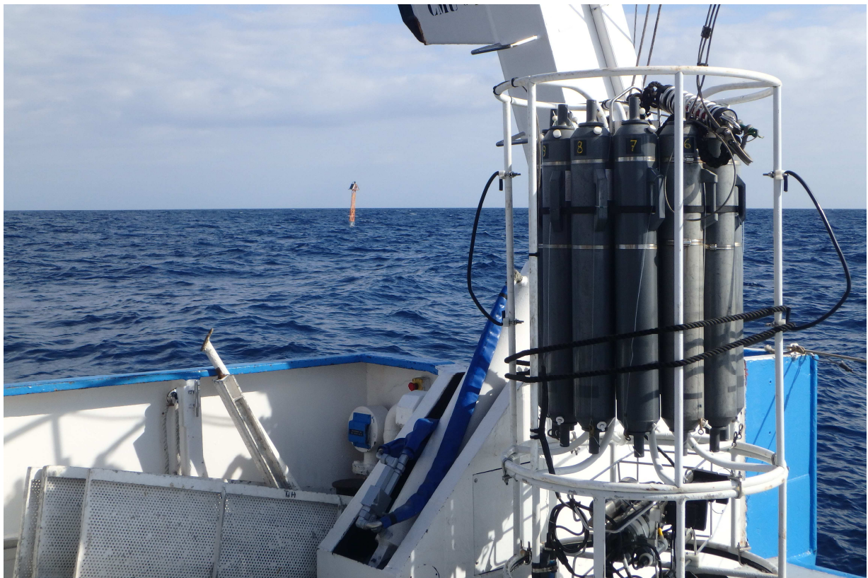
CTD Rosette on the deck of the R/V Téthys II before its deployment, and the BOUSSOLE buoy in the background.
